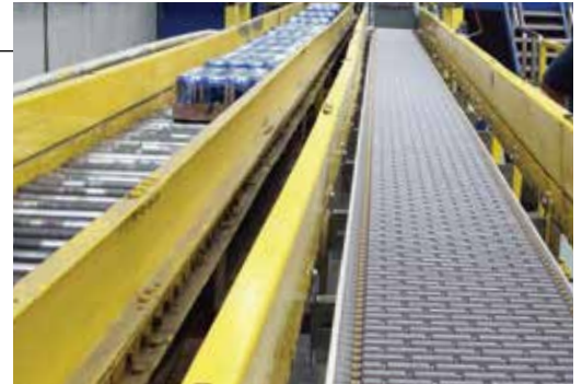
After: completed upgrade to Rexnord MatTop Chain
